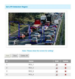
[Set LPR Detection Region]: You can set up to 4 ROI areas by drawing the screen. If you choose Normal Mode, it supports configuring the LPR detection regions for the current area. If you choose Advanced Mode(Only for PTZ series), it supports configuring different LPR detection regions for different PTZ presets(Only support Preset 1~4 so far).
